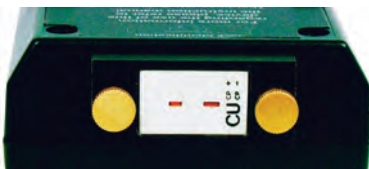
The TC-100 accepts both Mini-plug AND bare thermocouple wires
